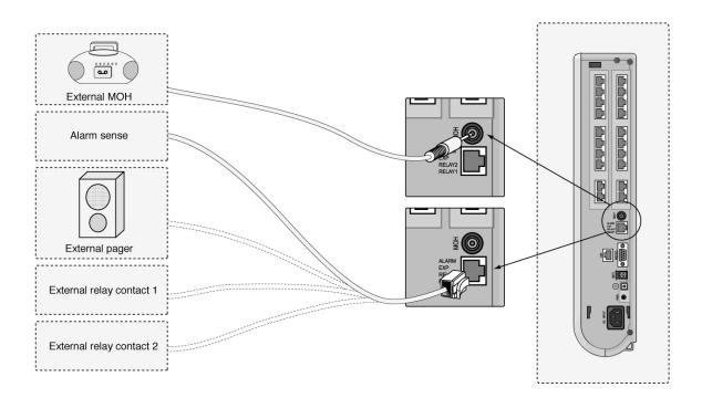
Figure 5.4.1 Additional Terminal Connection
